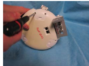
9.Six screws must be removed so the the back cover can be detached
