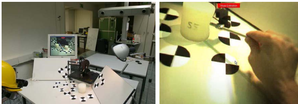
Figure 2-32 HMD augmented reality. Left: The major components of the system (Optotrak in background, the PHANTOM, the lamp, the landmarks placed on three different planes to cover the user's field of view involved in the system) Right: The stylus interface used to manipulate virtual objects. Images taken from [157].
