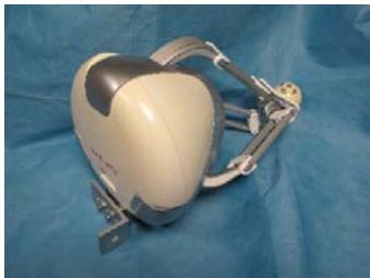
7.A Novint Falcon with a 90 degree rotated mount is shown here
