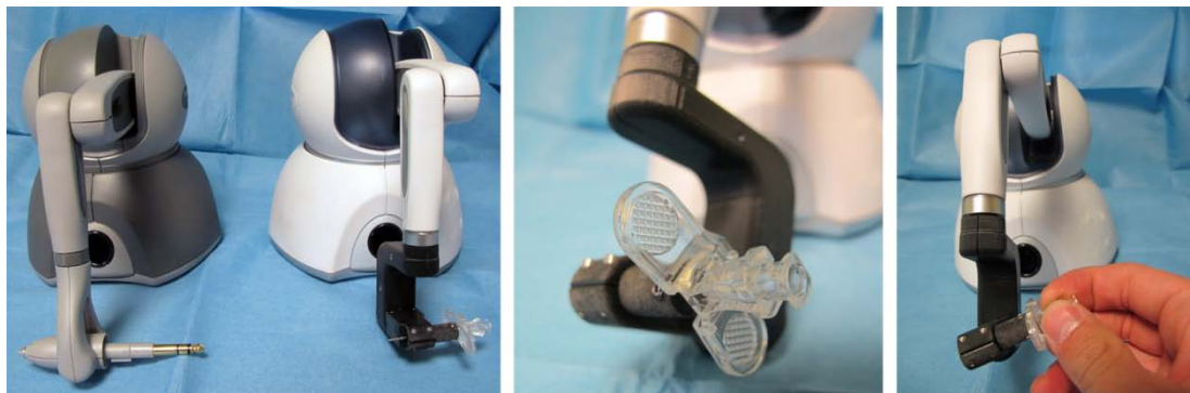
Figure 6-14 Left: A visual comparison of the off the shelf Omni with stylus removed and modified end effector. Centre: The needle hub mounted within the Omni end effector, providing high fidelity visual and tactile feedback as grasped. Right: The modified Omni as gripped by a user.
