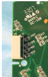
10.The eight pin connector leading from the end effector is labeled P2
