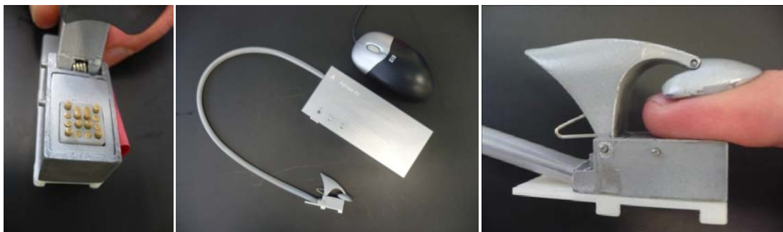
Figure 5-6 Finger mountable pin array device developed at Salford University [194].
