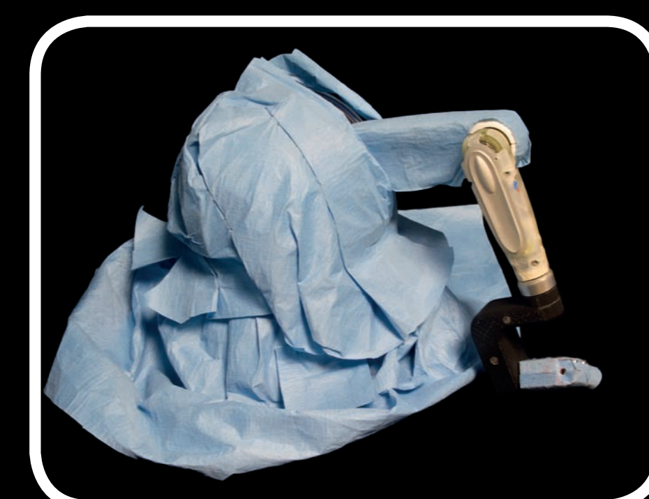
The arms two covers can now be re-attached, replacing the five screws and bolts. The arm is then covered in fenestrated drape for AR visualisation.
